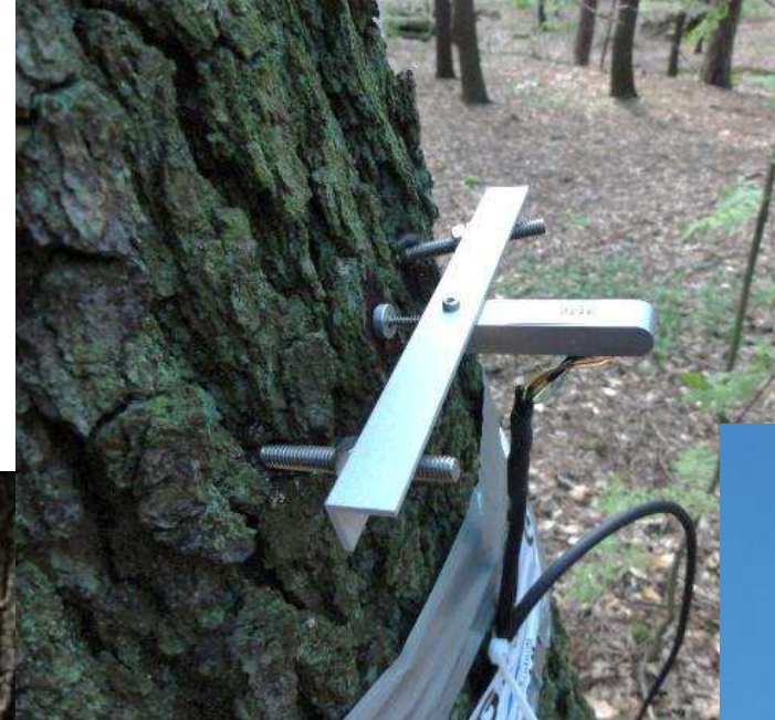
Point-Dendrometer (Wood growth)
