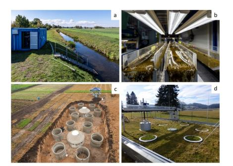
**Figure 2.** Examples of some of the TERENO experimental infrastructures: (a) MOBICOS container at an agricultural river side, (b) linear flumes within a MOBICOS container, (c) construction of a SoilCan lysimeter site, and (d) robotic system to measure soil greenhouse gas exchange on SoilCan lysimeters. Image sources: (a)–(c) André Kuenzelmann and UFZ, (d) TERENO.
