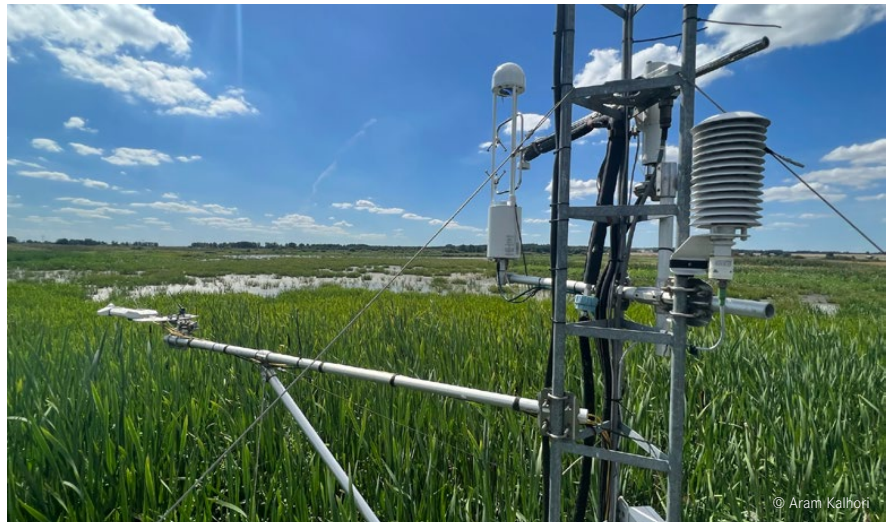
Measuring devices in the Polder Zarnekow record CO 2 and methane emissions in the peatland area. © Aram Kalhori
